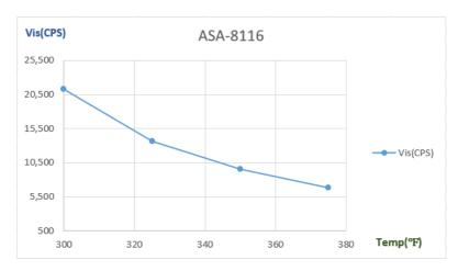
Viscosity 300°F~375°F (ASTM D3236, Brookfield RVDV-II+PRO, Spindle #27)
